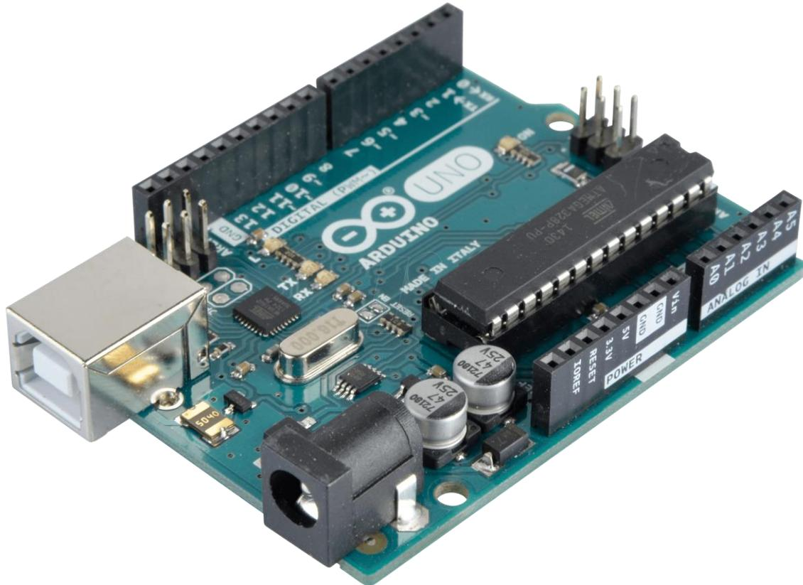
The Arduino PCB has an open source microcontroller on which someone could program, even if he is novice, in Windows, Linux and MAC OS X operation systems. The Arduino has I/O's (inputs, outputs) on which several components and peripherals could connect (Led, potentiometers, relay, sensors and many more) to provide us data (like temperature sensor) or for us to set data (e.g. LED On).
